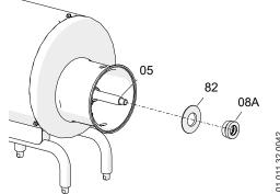
3. Place the splash ring (82) and the stationary part of the double mechanical seal (08A) on the shaft (05).
